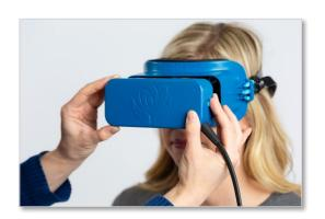
2. Press the camera unit onto the body unit with even and firm pressure. Confirm the camera unit is securely attached on both sides by ensuring that the camera unit does not move before proceeding with further use.
