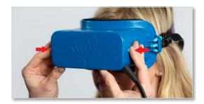
2. Remove the camera unit by pulling it straight away from the body unit.
