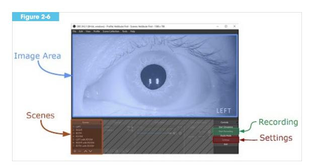
The main interface of OBS can be broken down into four main sections: Image Area, Scenes, Recording, and Settings.
